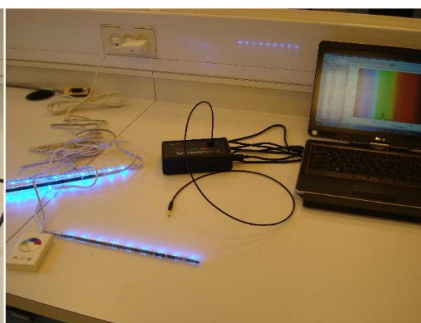
Emission measurement. Spectrophotometer with optical fibre unit and cable connected to a computer with LoggerPro.
