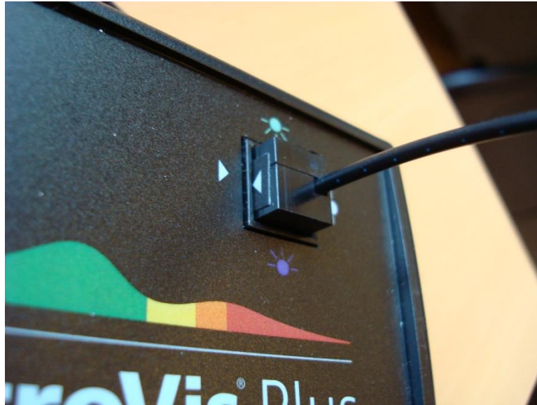
Figure 2.1b. Close-up of fibre unit mounted for emission measurements. Note the matching arrows.
